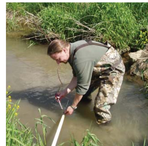
MCD staff installing the water quality sampling equipment in the Klase Ditch upstream of the construction.
